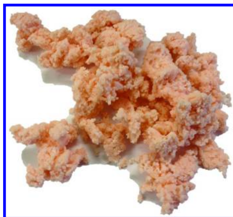
Figure 6. Image of a poly(styrene- b -AESO-styrene) triblock copolymer: Reproduced with permission from reference (32).
